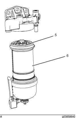
Illustration 84 Typical example **9.** Rotate the filter element (5) counterclockwise and remove the filter element . Clean the filter bowl.
