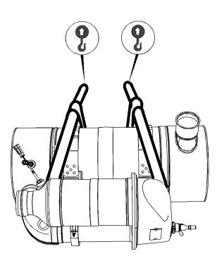
There are two sizes of CEM that can be installed. A high powered CEM and a low powered CEM. The approximate weight of the high powered CEM is 47 kg (104 lb), the approximate weight of the low powered CEM is 42 kg (93 lb).
