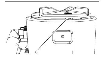
Illustration 73 Typical example **6.** Install the cap (1). Rotate the cap by hand clockwise until the cap locks into the locked position C on the breather body.
